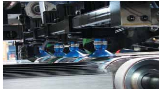
General view of front sucker cylinder carriage assembly
