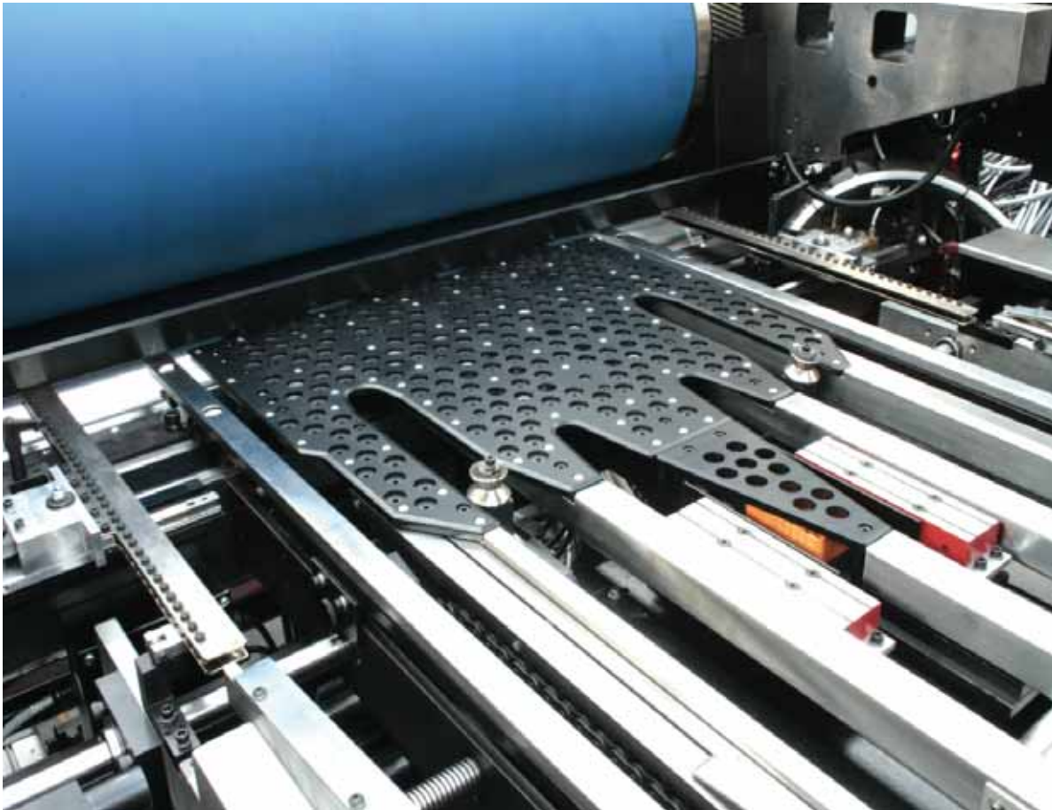
View showing extended plastic top plate on Fastready Gen3 Press Infeed
