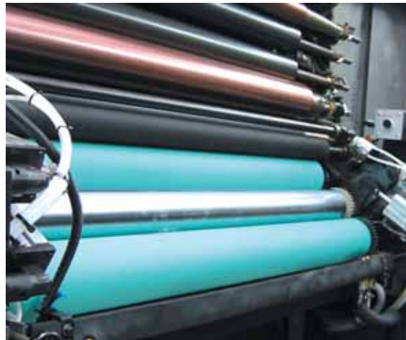
View of Delta ® Dampener fitted to a Marquess Press
