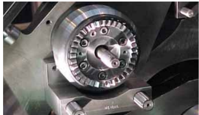
View of Anilox roller quick release coupling
