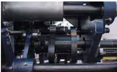
General view showing conjugate cam assembly for feed carriage
