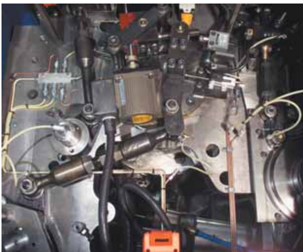
Above: View showing motorised stock thickness assembly fitted to Marquess Press
